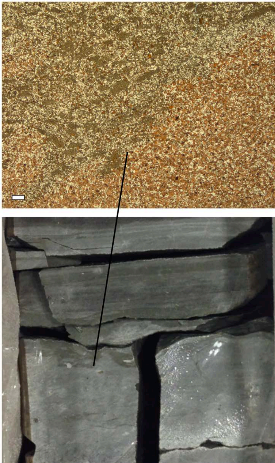
Figure 21. Photomicrograph and core photograph of firmground showing erosional relief and rip-up clasts, Tully core, 6805'. Scale bar is 0.5 mm.
