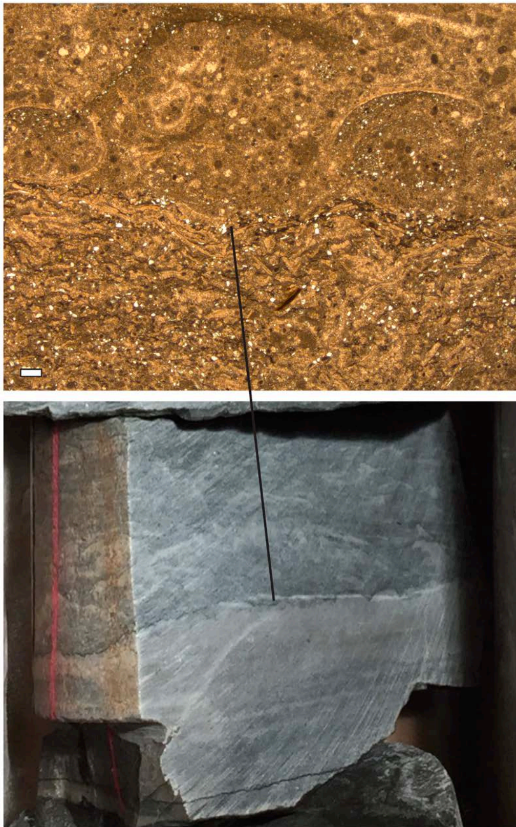
Figure 22. Photomicrograph and core photograph of firmground showing erosional relief, Tully core, 6809.7'. Scale bar is 0.5 mm.
